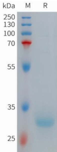
Figure 1. Human HAMP(65-84) Protein, hFc Tag on SDS-PAGE under reducing condition.
